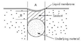
Correctly executed angle joint dimension A,B min. 6mm
